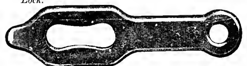
Fig. 2745. Stationary Seal-holder. PARTS OF FREIGHT-CAR DOOR-LOCK.
